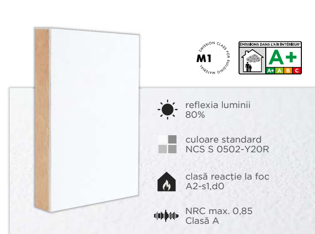
Fade™ Duo Systems Fade™ Acoustic board + Duo Primer + Duo Top
