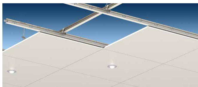
Renovated ceiling - concealed system
